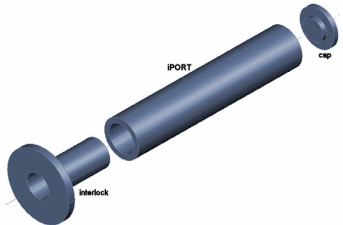
Figure 1: Assembly of interlock, iPORT and PMMA cap
